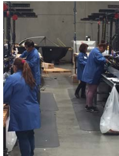
Figure 5: ESD Protection Measure during fixture assembly
