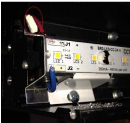
Figure 3: Broken Connector to LED Board
